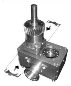
9. If clearance A does not correspond with these values, add or remove a shim.10. When the clearances A and B are within their limits, tighten all bearing cartridge bolts.11. Disassemble the rotors.
